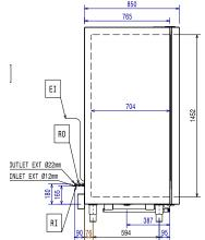
Drain Electrical inlet (power) RO Refrigerant Outlet
